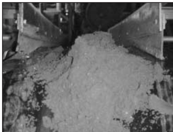
Dewatered sludge cake
